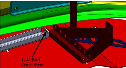
9. Install the 7 Clip Nuts in the existing holes along the bottom of the splitter as shown here
