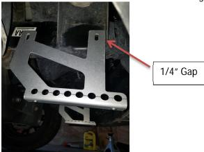
3. Once you have it where it needs to be, Mark the hole with a marker in the middle of the Oval Slot. This will give you some adjustment to make any final tweaks when bolting it up.
