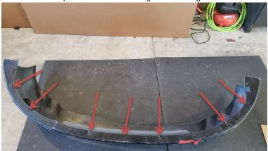
10. Adjust the brackets so its level with ground and at the same height as the bumper and Tighten all the bracket bolts. Have a friend help you hold up the splitter while you bolt it up to the brackets, leave the splitter bolts loose. Now, insert the 4 Plastic spacers provided on the outer ends. The larger one is the rear and the short one goes in front. Use the Large bolts with washers provided. Leave all of the screws loose
