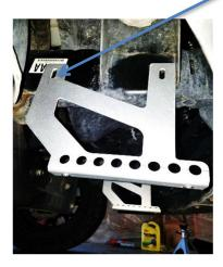
6. Now for the hole in the front Vertical Leg, Insert the Bolt with the washer and through one of the Hole in the bottom of the frame rail, insert the Nut. This can be a little tricky unless you have skinny fingers, Use a wrench to hold the nut by putting some tape on the nut so it doesn't fall off.
