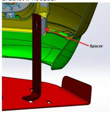
8. Install the Cross Member with 2 bolts and nuts provided as shown. The cross beam goes in between the 2 brackets.
