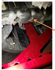
7. The outer brackets will now need to be installed. Remove the Bolt (18mm socket) on the bottom corner of the fog light bracket and insert the spacer in between the new bracket and the bumper with the leg pointing inwards and put the bolt back on. Use the new Carriage bolt provided. The bolt should be centered to the oval slot on the bracket. Adjust the height of the bracket if needed.
