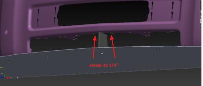
**STEP 3**Bolt up the splitter to the bumper using the 3/8" bolts and the 2x m6 screws as shown
