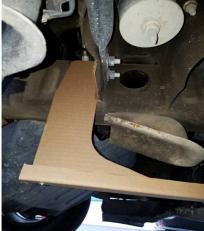
3. Remove the bolts on the outer ends of the bumper brace/strut and install the small brackets with lower leg facing back. Re-Use OEM Bolts.
