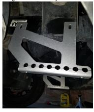
3. Once you have it where it needs to be, Mark the hole with a marker in the middle of the Oval Slot. This will give you some adjustment to make any final tweaks when bolting it up.
