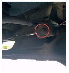
2. With the bumper off, remove the plastic valance and ALL of the plastic clips along the bottom of the steel bumper.
