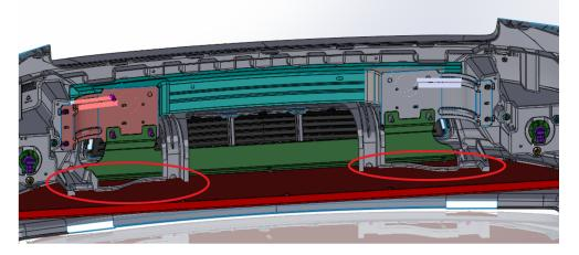
STEP 5: INSURE ALL BOLTS ARE PROPERLY SECURED AND TIGHTEN
